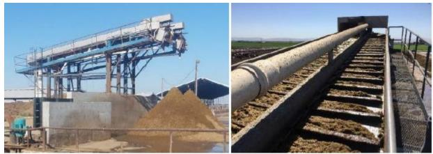
Source: <u>http://www.albersdairyequipment.com/manure.php</u> & (Edalati et al., 2019) Figure 2-2. Horizontal drag flight conveyor separator.
