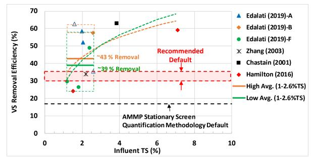
Figure 2-16. Recommended Quantification Methodology default for sloped screen separators
