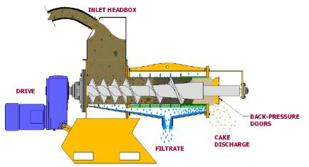
Source: Press Technology & Manufacturing: <u>https://www.presstechnology.com</u> Figure 2-5. Screw press schematic
