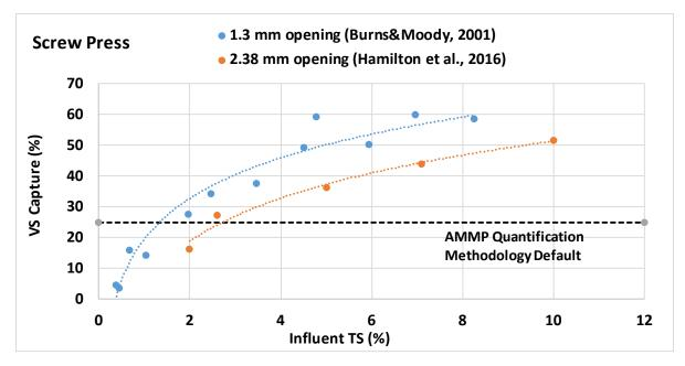
Figure 2-17. Volatile Solids removal versus Influent Total Solids Concentration; screw press.
