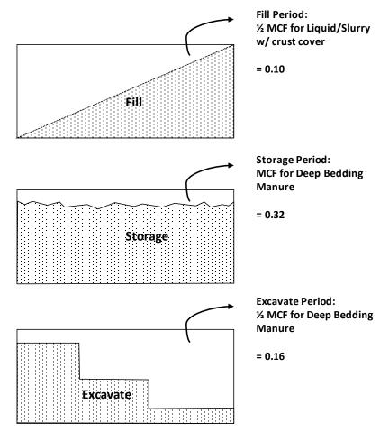
Figure 3-4.Representation of effective methane conversion factor fill, storage, and excavate phases of the weeping wall cycle
