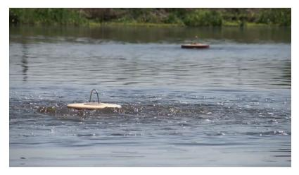
Figure 4-1 PondLift circulation device in a lagoon
