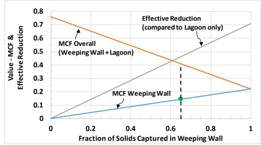
Figure 3-5 Effective weeping wall and overall methane conversion factors versus fraction of solids captured.
