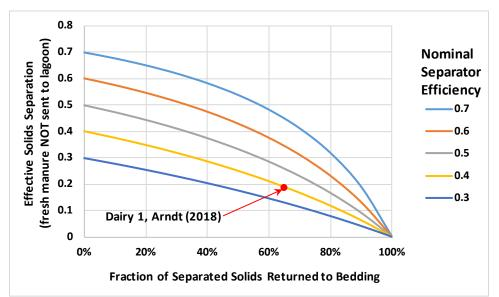
Figure 2-12. Effective separation versus fraction of solids returned to bedding.
