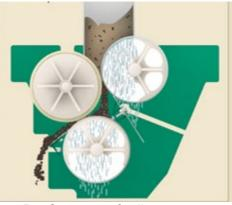
B. Cutaway of roller press Source: www.htequipment.net/Houle-Manure%20Separators.pdf
