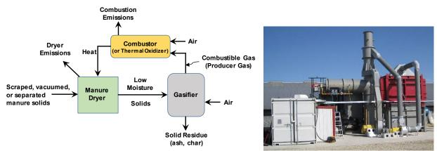
Figure 5-2 Schematic and photo of the Coaltec gasifier-close-coupled-combustion system.
