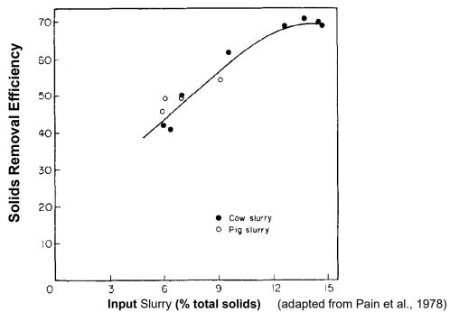
Figure 2-13 Relationship between input total solids and solids removal efficiency for a rotary screen separator
