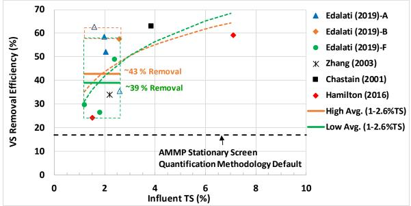
Notes: Orange dashed line is ln(x) curve fit of all data. Green dashed line is ln(x) fit of data after removing Edalati (2019)-A high and low. Dashed boxes indicate data for typical flush manure (influent TS  $\leq$  2.6% for this data). High average (43%) represents average of all data for influent TS  $\leq$  2.6%. Low average (39%) excludes the Edalati (2019)-A high and low.
