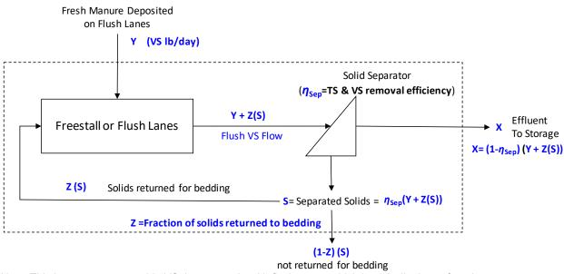
Note: This ignores any separable VS that comes in with flush water, which is typically drawn from lagoon storage.
