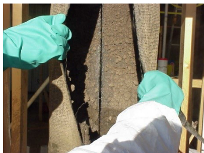
Dewatered dairy sludge
