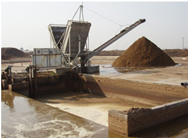
Figure 4–89 Temporary storage of mechanically separated solids in a conical pile below a stacking conveyor with windrows for longer term storage in the background
