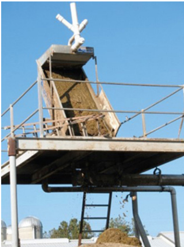
Figure 4–6 Schematic of a stationary inclined screen separator (Shutt et al. 1975; Virginia Polytechnic Institute, Virginia Cooperative Extension)
