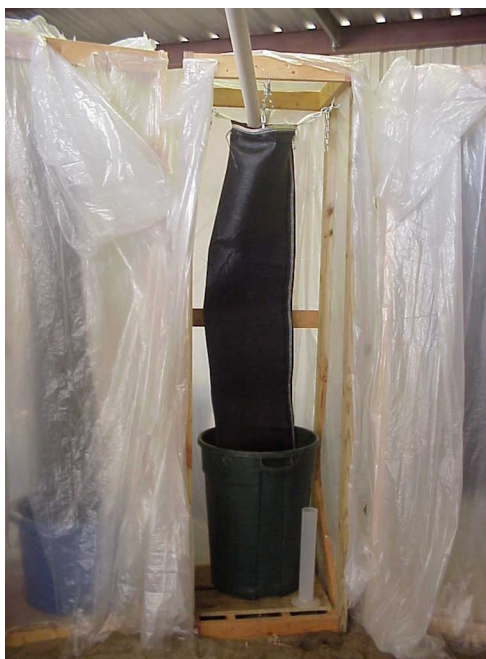
Figure 4–64 Test-scale geotextile tubes (Baker 2002)
